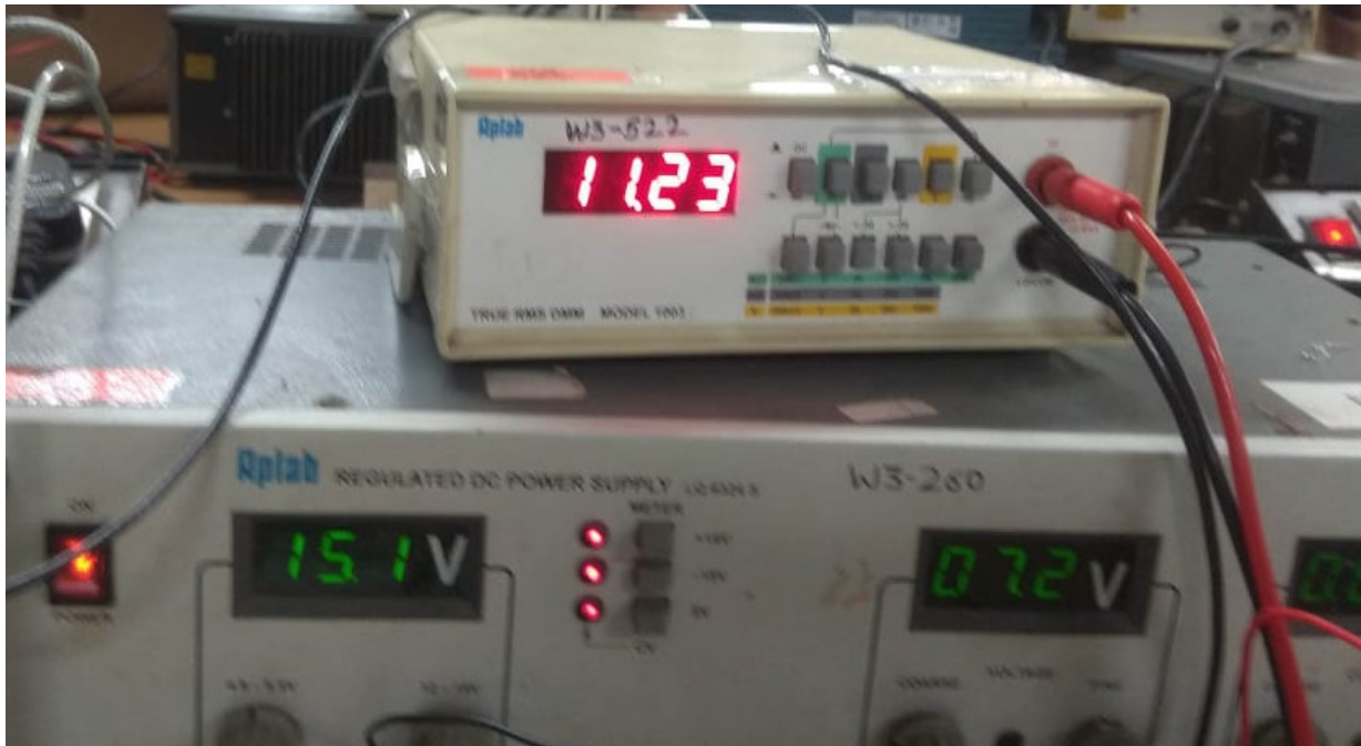
Figure 3.7: Input 7.2V , output 11.2V, duty ratio 0.4
