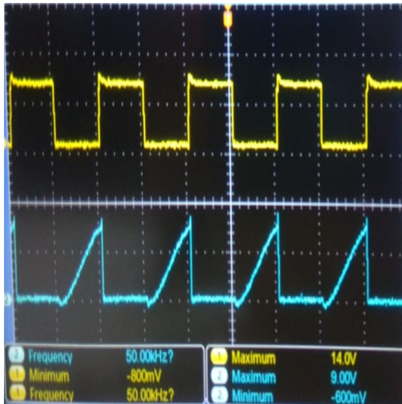
Figure 3.5: Input Signal and MOSFET Drain Signal not switching properly
