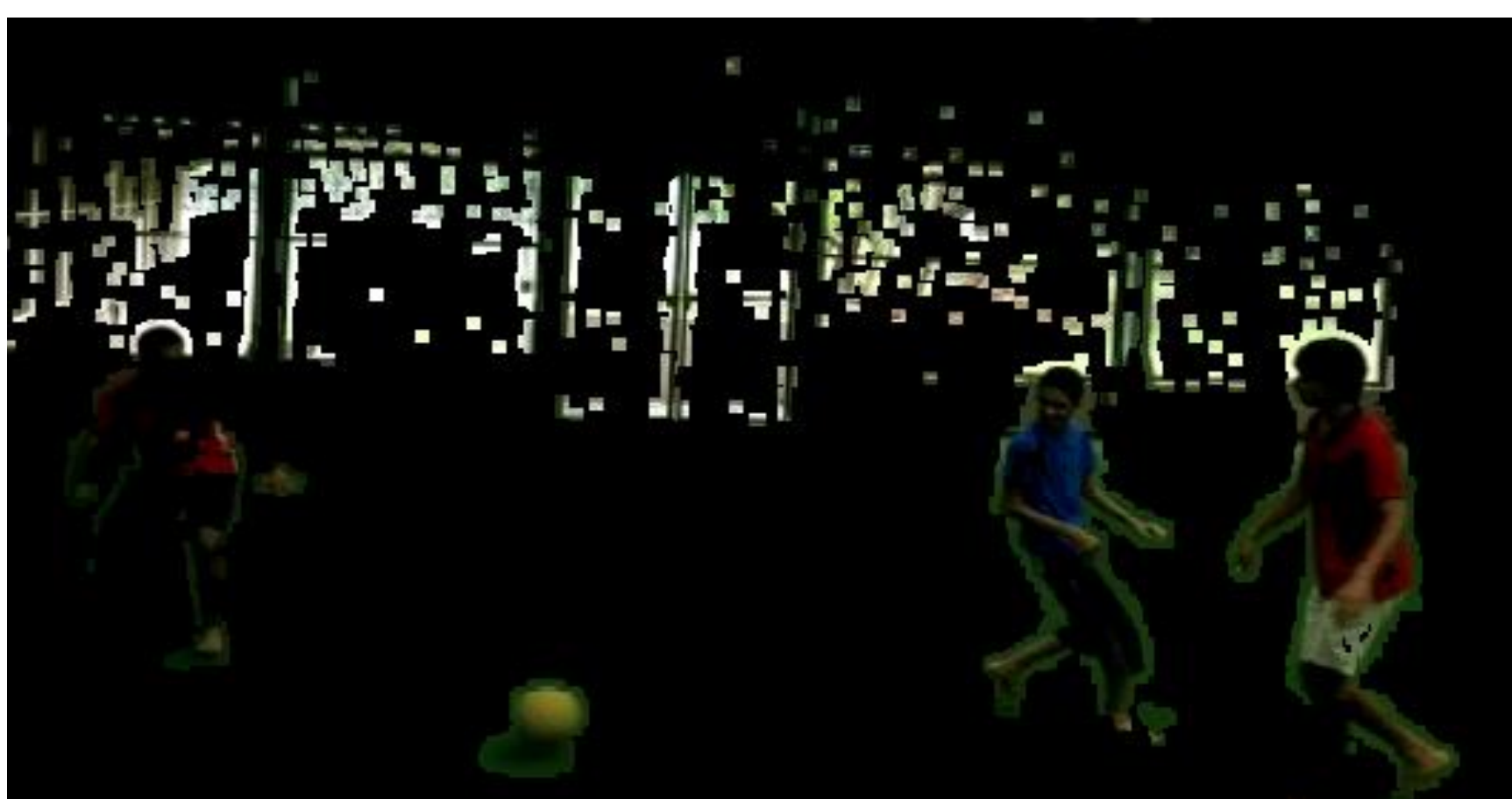
Figure 2: Image Processing in action! Seen here are the tracked elements with the pesky background subtracted
